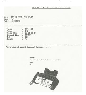
To use image TCR, the **Scan & Fax Mode** light must be on (press the button if necessary) and you must set these Menu options to On: Image TCR and Sending Confirm. See Scan & Fax Mode on page 29. Follow these instructions to set the menu options:
